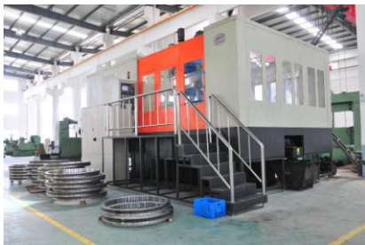
2.5m HIGH-SPEED CNC GEAR-MILLING MACHINE
